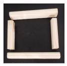
Now to make the counterweight box. Cut  $2 - 6\frac{1}{4}$  " pieces and  $2 - 3\frac{3}{4}$  " pieces which will become the frame for the counter weight box.
