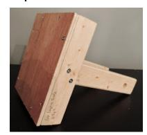
Finally use the 6" by 6" thin board to create the base for box and use the smaller screws to attach it.
