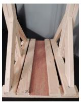
Take 2 - 16" lengths of 1 x 2 and a 2" by 16" piece of flat board and construct as seen.
