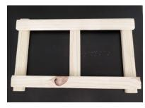
Create the base of the trebuchet by gluing together the 16" pieces' length wise on top of the 10" pieces. Add the 9" pieces in the middle and at each end. It should look like this...
