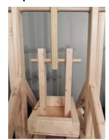
Attaching the counter weight bucket. Using the same method as with attaching the swing arm to the uprights, attach the bucket through the hole that was 1 1/2" from the end of the swing arm remembering where to place the rubberbands to lock it into place.
