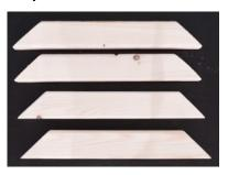
Cut 4 - 10" pieces with a 45 degree angle cut as shown below. Glue and screw them into place. These are the braces for the supports.
