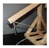
Tie one side of the finished sling through the hole on the main arm as shown.
