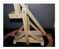
Bring the main arm down to the base. Measure the distance it takes to extend the slings to the back of the base. Make sure the sting is tight at the furthest point.
