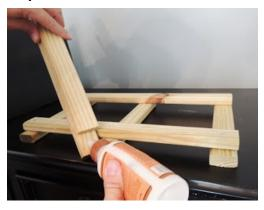
Glue the supports in place, and screw also them into place for added support (It is helpful to have the 12" dowel in place between the two supports to ensure proper placement)
